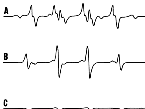
Fig. 5. ESR spectra of DMPO spin adducts obtained by 60-s irradiation of aqueous suspensions of powdery semiconductors. A: \text{CdS} , B: \text{WO}_3 , C: \text{Fe}_2\text{O}_3 , receiver gain: \times 100 (B), \times 200 (others), irradiation wavelength: 420 nm.
